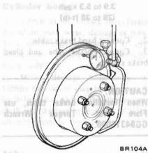
Fig. BR-34 Measuring Runout
