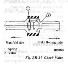
When installing check valve, be careful to avoid incorrect connections. See Fig. BR-37.
