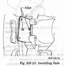
adjust brake pad-to-rotor clearance. Clearance is correct if brake pedal stroke is constant.
