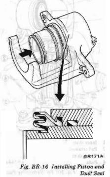
4. Coat the following part with recommended brake grease. See Fig. BR-12.
