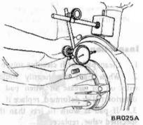
Fig. BR-17 Measuring Runout
