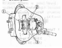
88094A Fig. BR-20 Removing Pads
