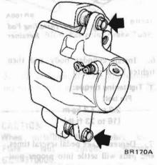
Fig. BR-15 Removing Pin Bolts
