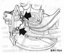
Fig. BR-24 Removing Caliper Long Life -----
