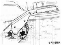
Fig. BR-44 Removing Control Lever
