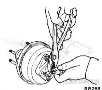
Fig. BR-41 Adjusting Push Rod Length
