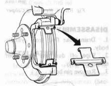
BR168A Fig. BR-13 Installing Pad Retainer
