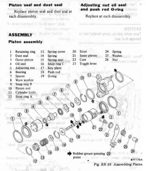
Assemble piston assembly in the reverse procedure of disassembly, paying particular attention to the following:
